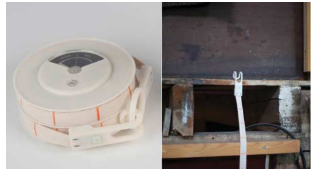
Figure 11. The Temperature Tape with fabric tape striped with thermo chromatic ink, a needle dial and hooks on either of the fabric tape (Cameron et al. , 2014). ©Interaction Research Studio, Goldsmiths.
