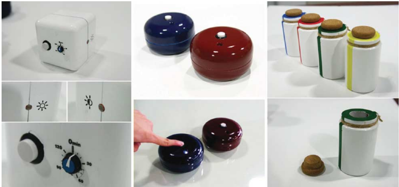
Figure 1. The Discovery-Driven Prototypes (Lim et al. , 2013) consist of three artifacts: (from L to R): Aeng-aeng-ye is a music timer; Deol-deol-ye is communication device and Tong is a sound recorder.
